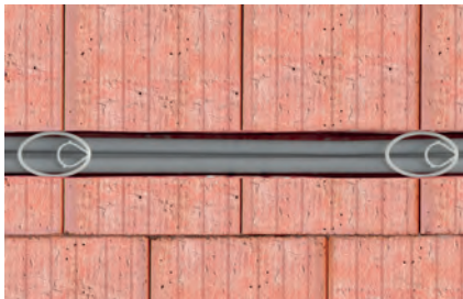
Cable fixing in wall slots > 30 mm
